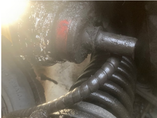
Figure 1: Pin end showing failed weld and exposed internal rod
