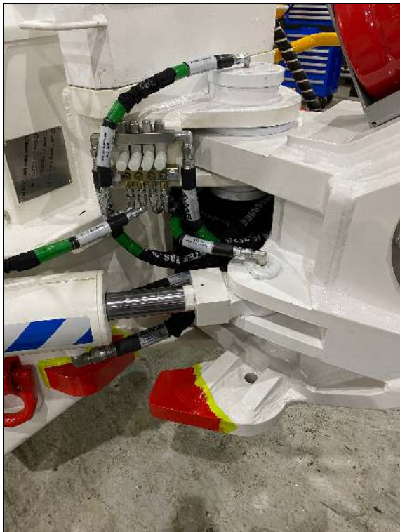
Figure 3: Upgraded Hitch Articulation
