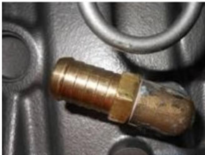
**Figure 1 – 3/8 BSP elbow installed in the drivers side of the engine block**
