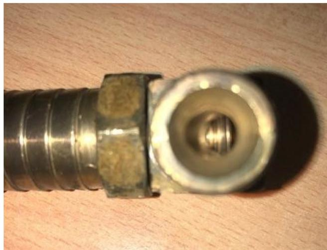
**Figure 2 – Alternate square drilled fitting**
