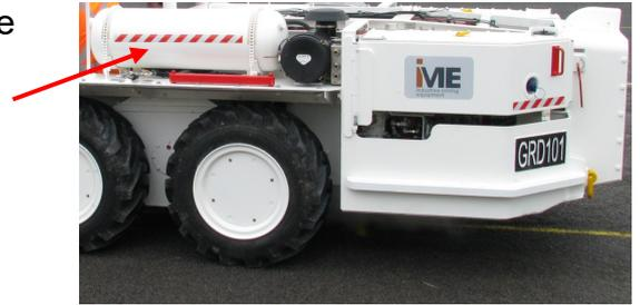
**Description:** The main air reservoir is filled via the charge point (below the main air reservoir), and mains system pressure flows to the main reservoir pressure gauge, and supplies the full pneumatic circuit, starting, and rear service brakes. The main air reservoir is isolated from the circuit by a main isolation valve, located in the driver's cabin at the entry.
