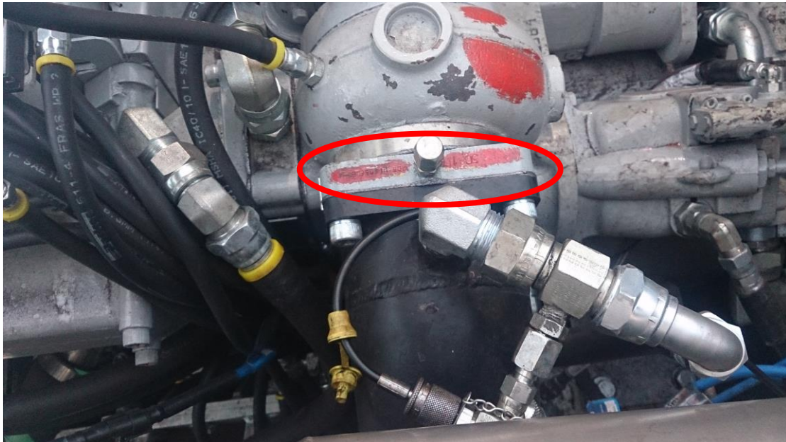
Exhaust adapter plate without heat shield installed
