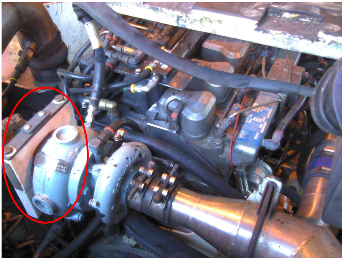
MWM Engine System with the Heat Shield Assembly P/N 7-055756-700 Installed
