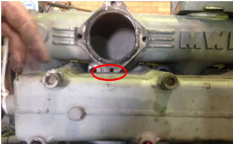
Failed Manifold with flange detached.
