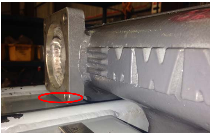
Inlet manifold flange & port chamber adjacent to exhaust manifold – Clearance should be observed in area indicated
